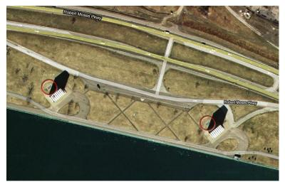
Not much security attention is given to the water inlets, but without these the dams are useless. A necessary structure for the sluice gates along the Niagara River are large air vents; the black objects in the red circles. These prevent vacuums from forming when the gates are closed, and also provide maintenance hatches.
